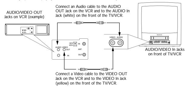
When all connections are complete, plug in the TV/VCR's power cord.
